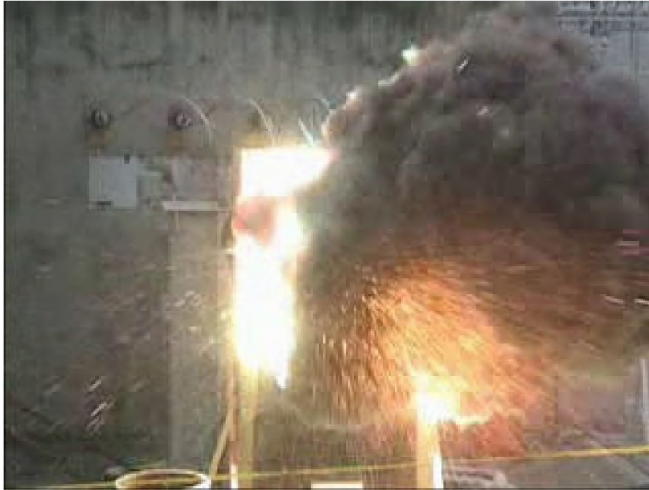
Arc Flash Hazard of 480 VAC Circuit Breaker Failure
